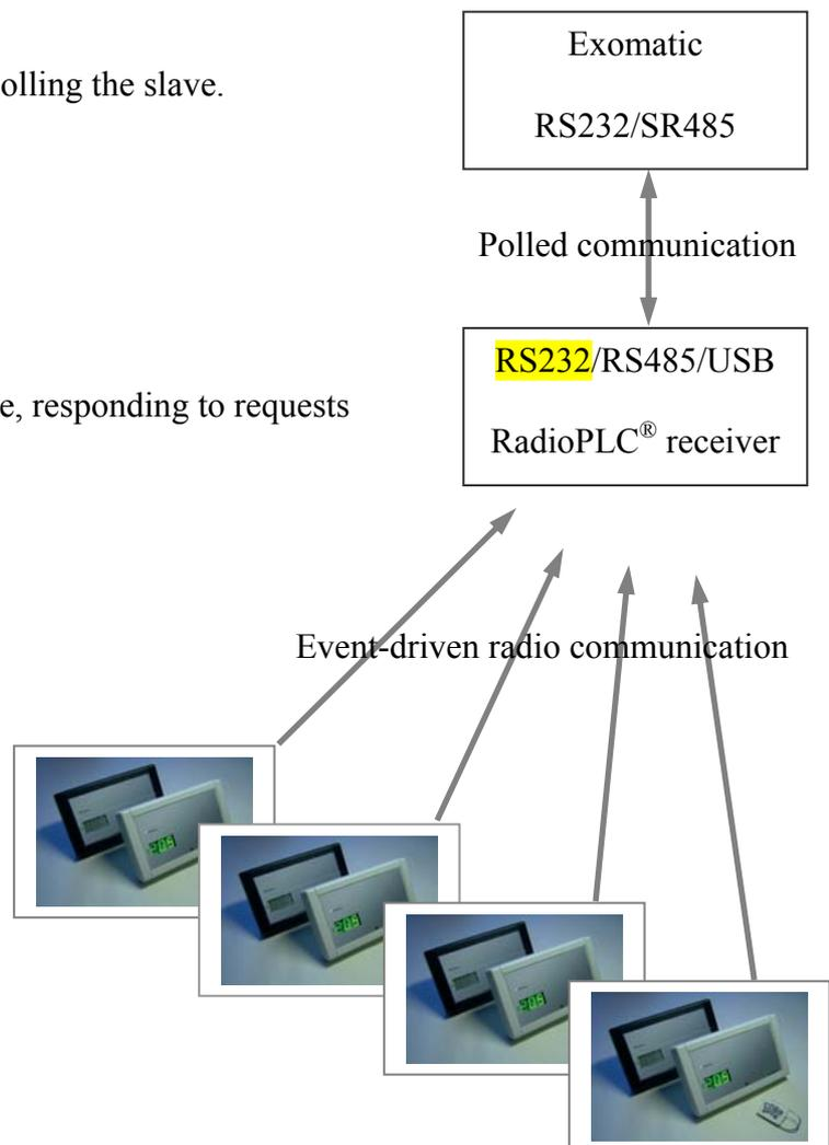
The ModBus communication might be possible to run simultaneously with the RadioPLC<sup>®</sup> terminal mode, thus simplifying test, setup and field service.
